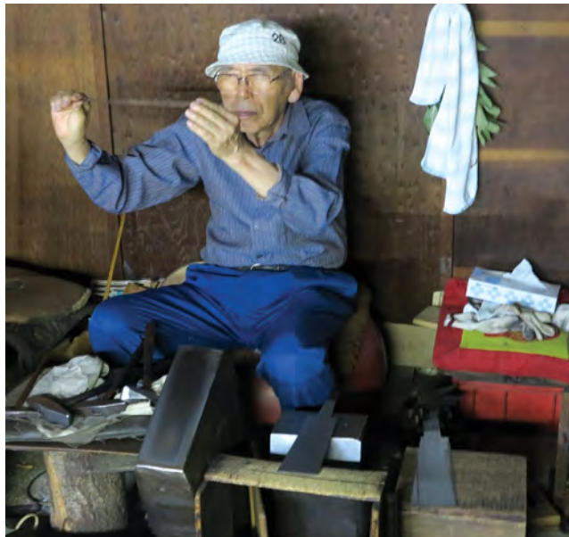
A master saw finisher at Hishika Saw Works checks a blade to ensure that it is straight and smooth.
